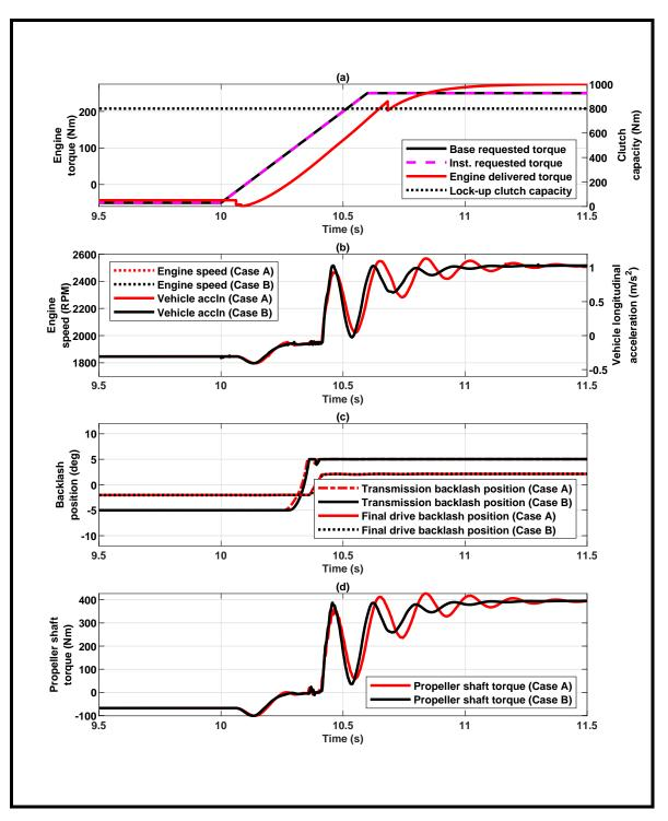
**Figure 3.13:** Effect of changing axle shaft stiffness on overall driveline response. Case A represents condition where axle shaft stiffness is increased by 25%. Case B represents condition where axle shaft stiffness is decreased by 25%.
