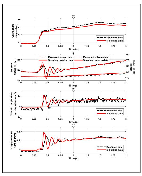
Figure 2.15: Results for sub-case 5of model validation: Comparison experimental simulation with between and data reduced coefficient of rolling resistance(Table 2.10.
