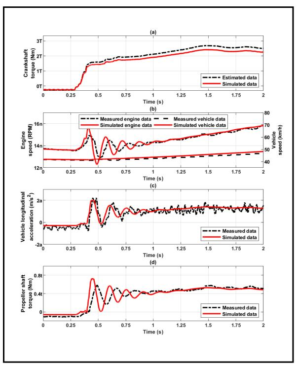
Figure 2.16: Results for sub-case 6 ofmodel validation: Comparison experimental simulation with between and data reduced axle and propeller shaft stiffness(Table 2.12).
