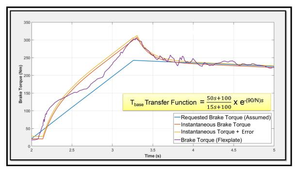
Figure B.2: Observed engine torque response for a throttle input of  $0 \rightarrow 60\%$
