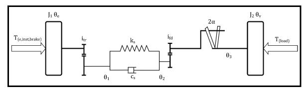
Figure 4.1: ROM with lumped tire parameters.
