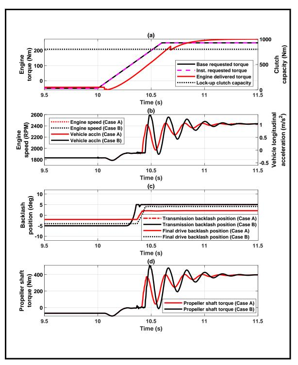
**Figure 3.11:** Effect of increasing the final drive backlash on driveline response. Case A represents condition where final drive backlash is 4 deg. Case B represents condition where final drive backlash is 8 deg.
