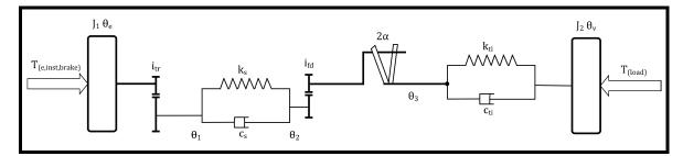
Figure 4.3: ROM with separate tire parameters.
