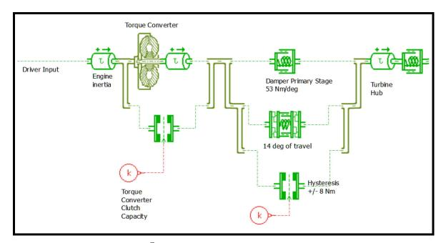
Figure 2.3: Amesim<sup> $\mathbb{R}$ </sup> model showing the torque converter with lock-up clutch and spring hysteresis blocks.
