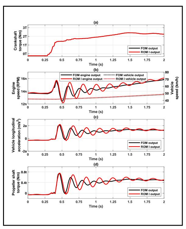
**Figure 4.2:** <u>Comparison of ROM I</u> with lumped tire parameters' driveline response with FOM, for a tip-in scenario.
