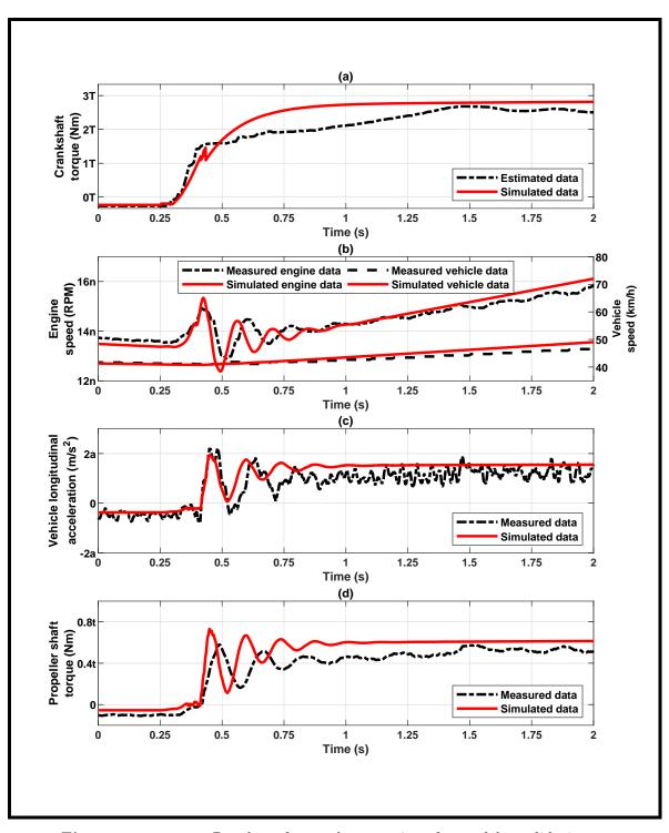
Figure 2.12: Results for sub-case  $\mathbf{2}$ of model validation: Comparison between experimental simulation with and data increased vehicle mass(Table 2.4).
