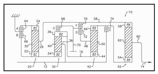
Figure 2.4: Schematic diagram showing the 10-speed transmission[14].
