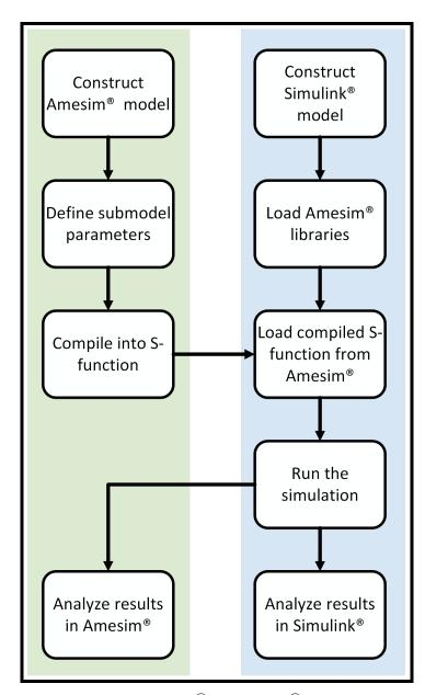
**Figure 2.2:** Overview of  $Amesim^{\textcircled{R}}$  -  $Simulink^{\textcircled{R}}$  interface. Adapted from [13].
