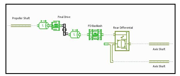
**Figure 2.7:** Amesim<sup> $\mathbb{R}$ </sup> model showing the propeller and axle shafts, along with the rear differential and final drive backlash.
