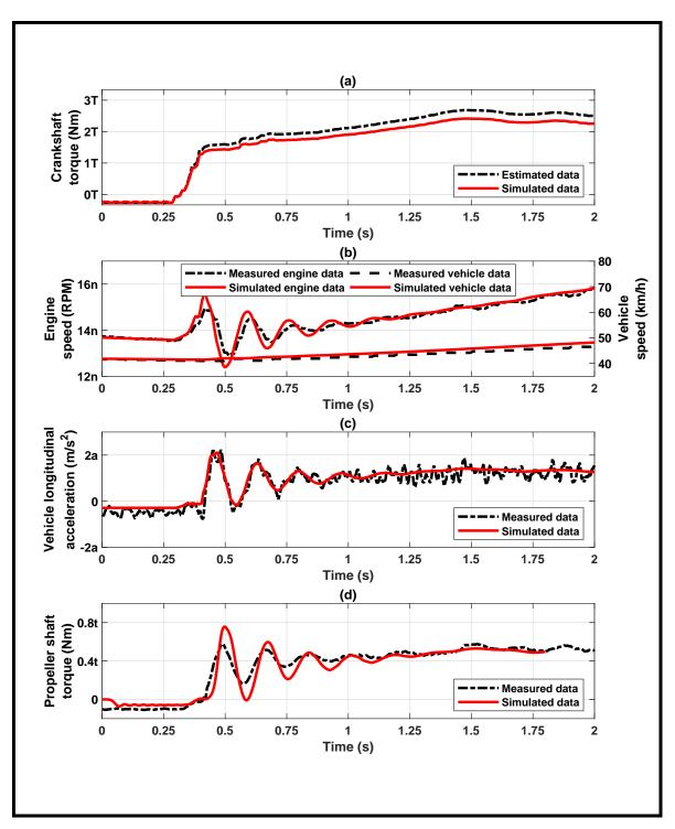
Figure 2.18: Simulation output in 5th gear with estimated crankshaft torque compensated for error as input to  $Amesim^{\textcircled{(R)}}$ , modified vehicle mass, modified coefficient of rolling resistance, modified propeller shaft and axle shaft stiffness, and modified engine, torque converter and transmission inertia, and filtered driveshaft torque.
