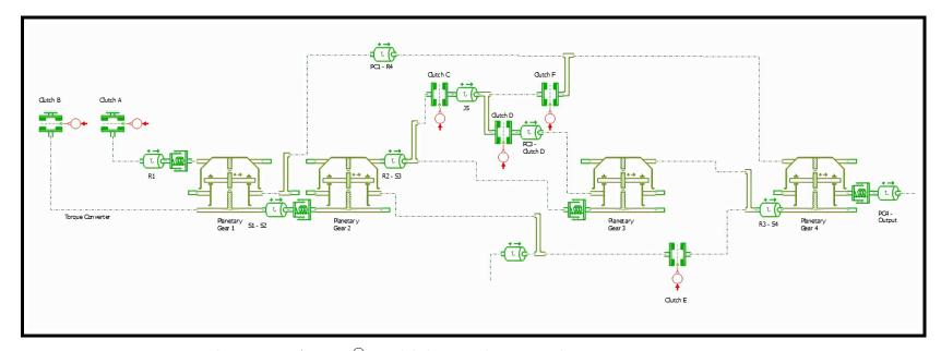
Figure 2.5:  $\text{Amesim}^{\textcircled{R}}$  model showing the 10-speed automatic transmission blocks.
