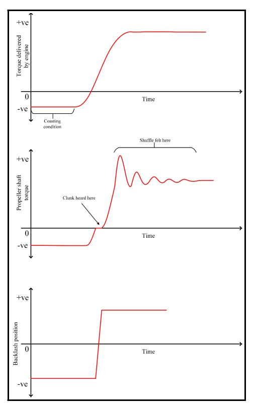
**Figure 1.6:** Representative output of propeller shaft torque showing clunk and shuffle, and backlash traversal in driveline.
