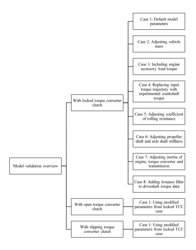
Figure 2.10: Overview of the model validation work done.
