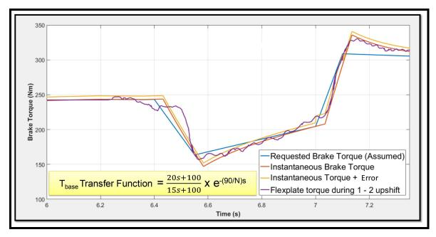
Figure B.4: Observed response for a throttle tip-out scenario
