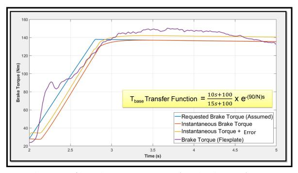
**Figure B.3:** Observed engine torque response for a throttle input of  $0 \rightarrow 20\%$
