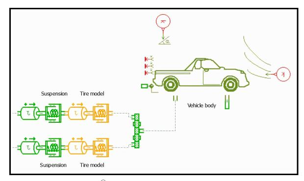
Figure 2.8: Amesim<sup>®</sup> model showing the suspension, tire and the vehicle dynamics blocks.
